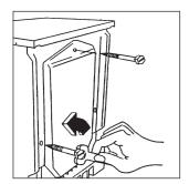
Unscrew and remove the three rear screws by means of a key.
